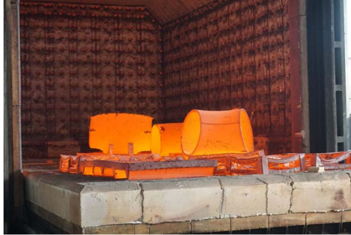
Figure 4 – Tempering the component in furnace
