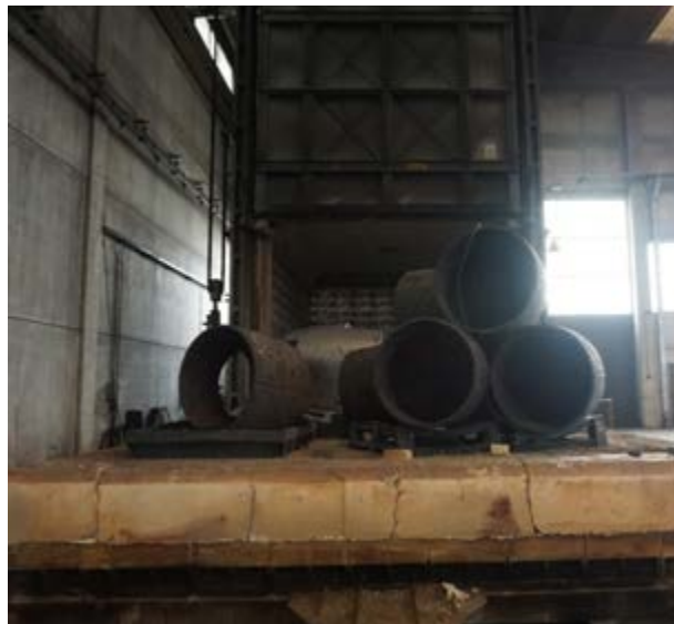
Figure 5 – Component is allowed to cool in still air
