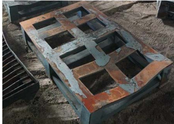
Figure 6 - Steel pallet used to support welded elbows in the furnace
