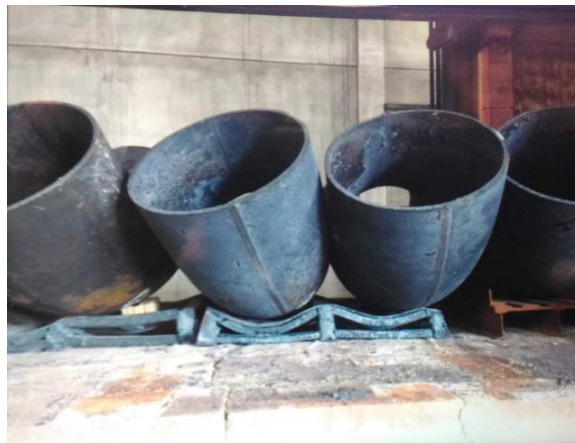
Figure 8 – Improper furnace loading simulation, areas of low yield strength on the elbows have been linked to where the fittings touch each other and the pallets on which they sit
