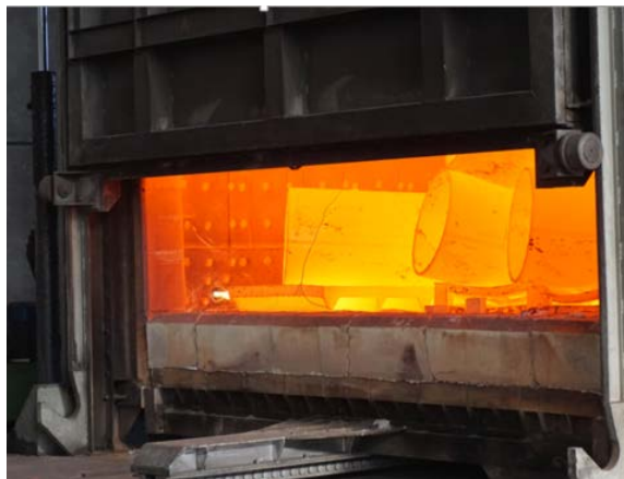
Figure 1- Heating the component to its austenitization temperature range for a specified amount of time
