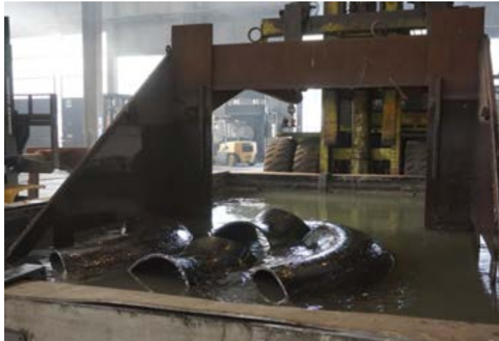
Figure 2 – Water quenching the component
