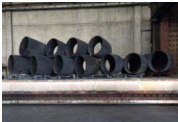
Figure 7 - Welded elbows placed in stacking arrangement
